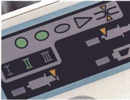
Three signals light up from left to right as infusion pressure rises.
